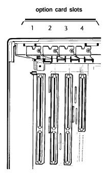
Slots 1 through 3 are designed for 16-bit option cards and slot 4 is designed for an 8-bit card. As you can see below, a 16-bit card has an extra connector along the bottom.
